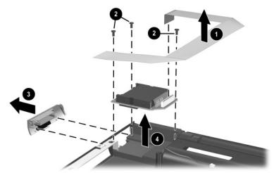
Removing the SD Card Slot/Infrared Module
